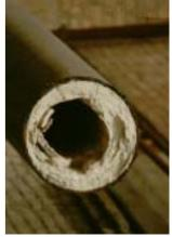
finely divided sludge. Vibrations of heating surfaces prevent deposition of the sludge on the pipe walls. Thus particles of insoluble salts do not reach the walls of equipment remaining in a suspended state and can be easily removed by the flow of water or air blowing.
